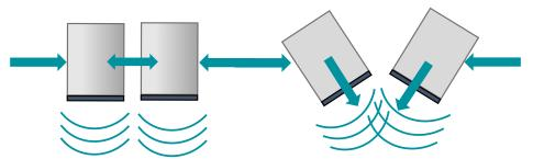
Lateral vibration is detrimental to the integrity of traditional cutting structures, but Ulterra's proprietary CounterForce cutting structure redirects the lateral vibration back into the formation, keeping the cutters sharper, longer.
